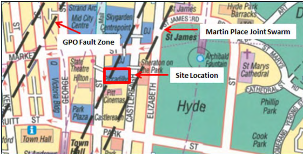
Figure 2: Near vertical structural features (adapted from Pells, Braybrooke & Och, 2004).
